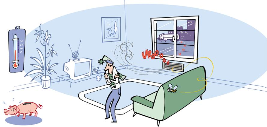
With the use of ventilation by thermal draft (so-called “natural” way), the outside air enters by grilles placed at the bottom of facade walls. The hot indoor air, being lighter than cold air, leaves by grilles placed in the upper part of the wall.
